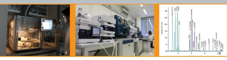
Automated sample preparation system (Biotage) for SPE, SLE, and PPT methods in 96-array format.
